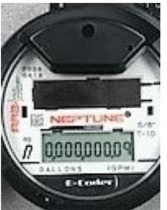
3. Write down the first set of numbers that come up. This is your reading. Most residential houses have a standard 5/8" meter. In this case, you only need to write down the first four numbers from left to right. In the above example, your reading would be 0000. Compare this number to the reading number on your current and previous bills.
