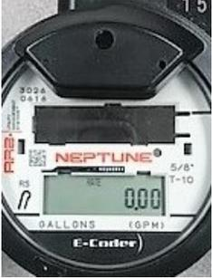
4. Then check your rate of flow. If your rate of flow is ANYTHING besides 0.00, then something in your house is running. It is most often a silent toilet leak. To test for this, put food coloring in the toilet tank and do not flush for approximately 90 minutes. If any of the coloring moves to the toilet bowl, then you have a leak. You may also hear the toilet running periodically, which is indicative of an intermittent leak.
