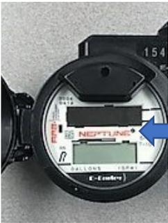
2. Shine a bright flashlight onto the face of the meter, focusing the light on the small circle in between the two screens as shown in the picture. This will cause numbers to pop up within a few seconds. If no numbers show, your flashlight may not be bright enough.
